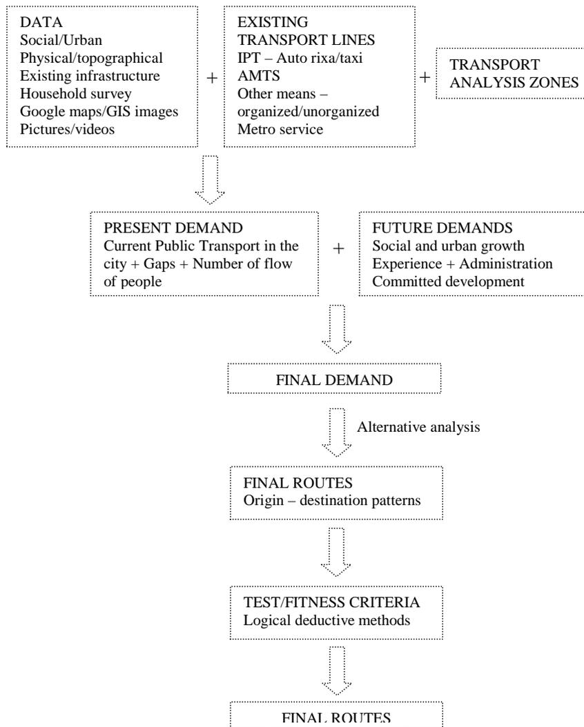
Figure 6. Design process BRTS, Ahmedabad using Emme 3 (Transport modelling engine)
